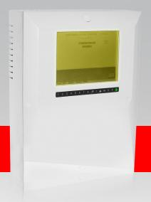
The IFS7002R repeater panel allows vital information from the IFS7000 system to be communicated through points around the building, remote from the fire alarm control panels. Distributed at strategic points in a facility - such as nurse stations, floor landings, control rooms - valuable time can be saved when identifying the location of a fire and evacuating the building.
