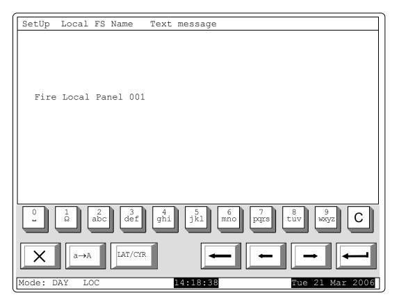
In *CAN Local panel name* select the option for assigning a name to the local object. The name of the local object is a randomly composed string and may contain letters and figures (up to 20). After reverting to the main menu you may continue the configuration of the local parameters.
