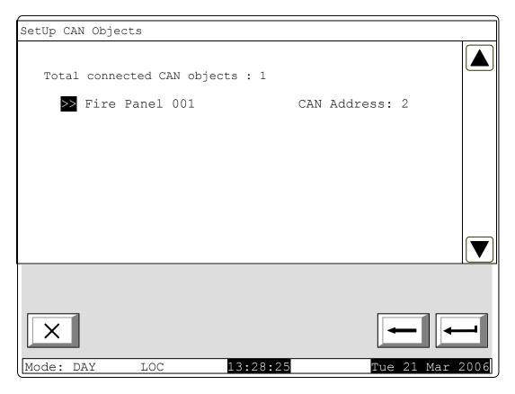
The menu above contains information for connected objects. Scroll down to select the desired object for configuration:
