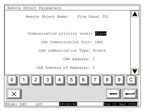
In this menu corrections can be make to an existing CAN object. The field *Communication Priority Level* defines the position of the described remote object (fire control panel) in the network – *Master* or *Slave*. The field *CAN Communication port* defines the port where the object is connected to. The connection type defines the means of the connection. In case of direct connection, the objects are assigned to one and the same CAN, in the address field of the
