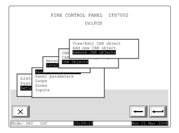
Select the option *Remove CAN object* to display the list of all connected CAN objects:
