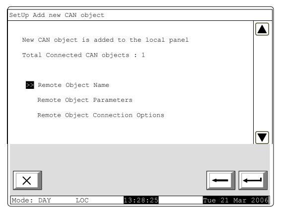
A name of the remote object can be assigned using the menu displayed above. The name is a random one (up to 20 symbols) and is not mandatory the same name given in the local parameters of the remote object.
