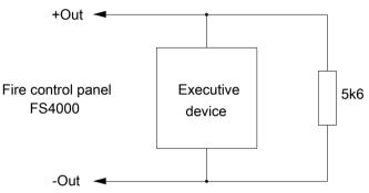
If the monitored output is not in use, fix a resistor 5k6/0,25W immediately to terminals "+Outx" and "-Outx".
