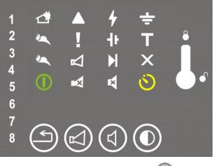
In Duty mode are active only the green LED indicator (1) (Power supply ) and the yellow indicator (3) if a delay is set for the outputs. The local buzzer is off.
