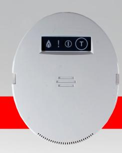
For detection of compressed natural gas (methane) in the protected area. The status is indicated with LEDs and built-in sounder. EN50194-1 compatible on trigger level 5100 ppm CNG (methane) in air, saturation 10% LEL (Low Explosion Level) of the protected area. The signal loop interface line is compatible with the IFS7002 fire control panel.
