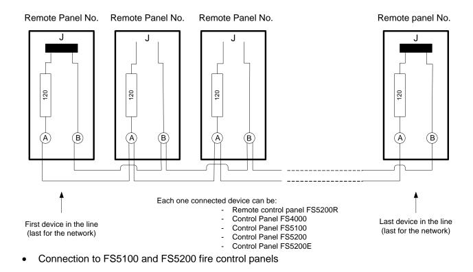
Interface PC board should be installed to the configuration of the fire control panels so that FS1200 and FS5200 could operate with a repeater.
