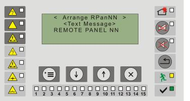
After the name is entered, all messages referring that remote fire control panel will be visualized and displayed with the name assigned by the user.
