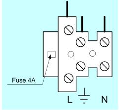
The cable should be with double-insulation and cross section not less than 0.5mm<sup>2</sup> for the power supply wires and 1,5mm<sup>2</sup> for the earthing wire.
