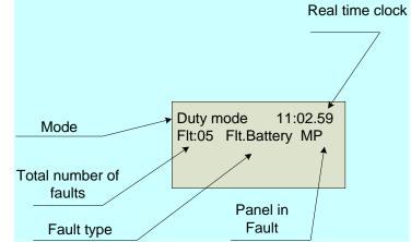
The most frequently indicated fault conditions in the repeater are:
