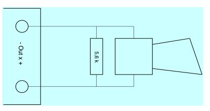
Voltage (24±3) V with load carrying capacity 1A is supplied upon activation of the outputs. The outputs are activated for Fire condition in the remote fire control panel.
