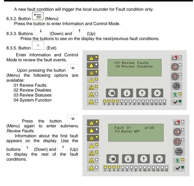
Press button  $[\times]$  (Exit) to exit the review of the faults.
